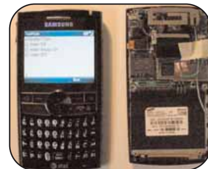
Figure 10. Prototype antenna installed in a production handset
