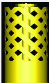
3-D model of the octafilar antenna in the MicroStripes build module. The dielectric core medium has been removed to reveal the entire metallized surface.
