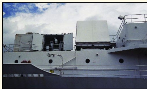
The US Navy's S-Band Mobile Array Telemetry (SMART) antenna, developed by Lockheed Martin, is used for missile telemetry tracking. The optics subsystem is shown at left and the phased array is shown at right.
